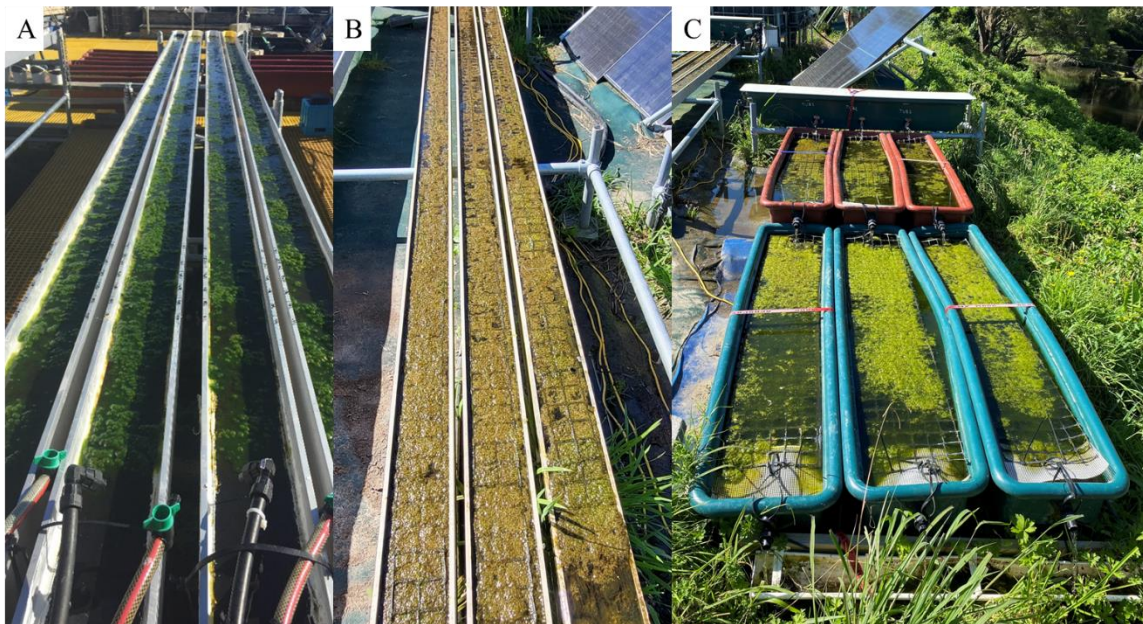
Figure 2: Three different FANS operation modes a) Attached, b) Shallow suspended and c) Deep suspended FANS.
