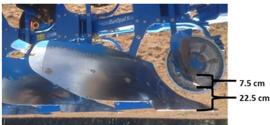
Figure 3. Skimmer share set 22.5 cm above mouldboard share point and 7.5 cm below the soil surface.
