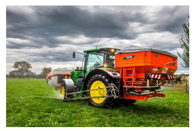
Fig. 2 Kuhn spreader mounted on John Deere tractor and modified for ONEsystem® and GA application
