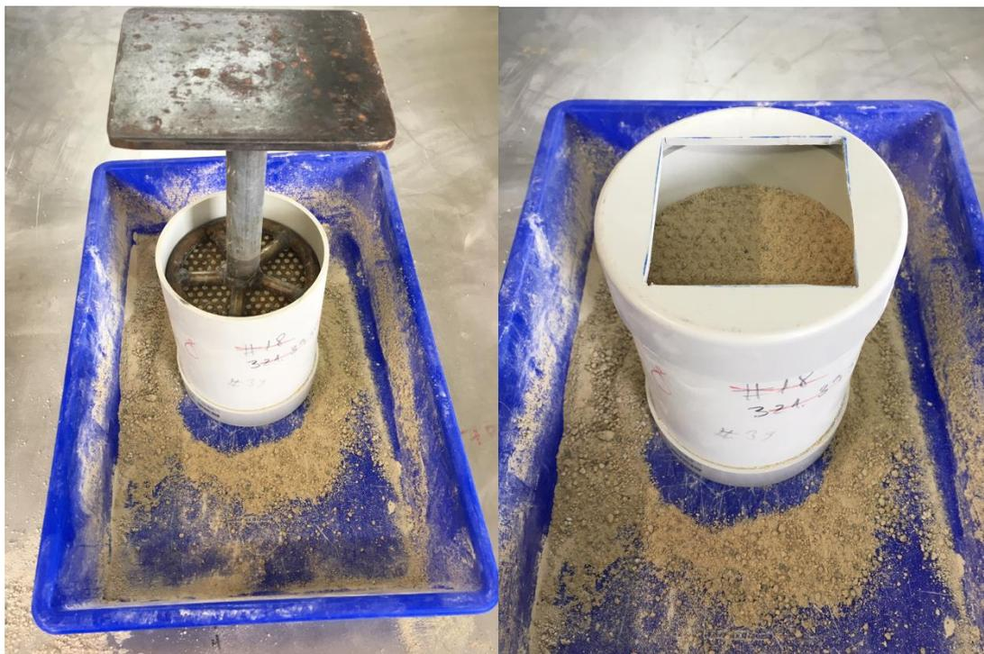
**Figure 3: After tapping the side of the cylinder at least 3 times to remove air, a porous metal tool (left) is used to press down on the lime, to simulate the weight of material above it in the hopper, then the amount the lime compresses is measured. The cap is then fit to the open end (right) for the bridging test.**
