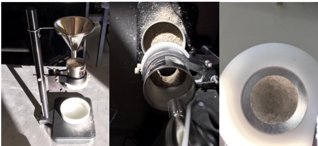
**Figure 2: Left – Flodex device; Center – lime sample passing orifice; Right – lime lodged inside (bottom view)**
