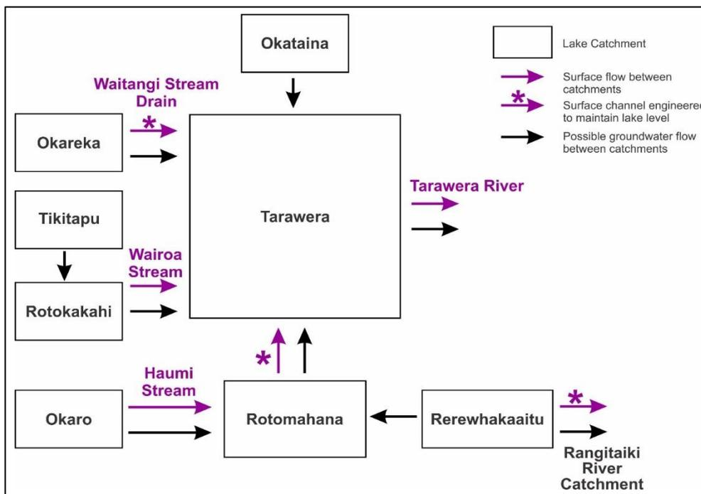
**Figure 2: Tarawera lakes hydrology schematic (from White et al, 2016)**
