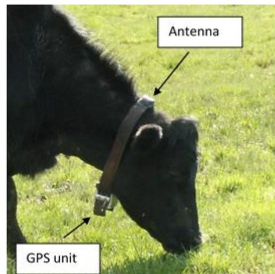
**Figure 2 Cow wearing GPS collar with antenna and GPS unit.**
