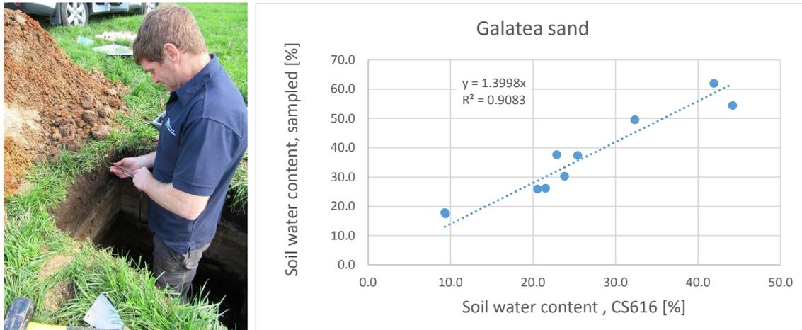
**Figure 4.** Scott Mahupuku from the Bay of Plenty Regional Council carries out a field calibration of a CS616 time-domain reflectometry (TDR) sensor (Campbell Scientific, USA) on Galatea sand. Steel cores were inserted beside the TDR waveguide to determine the soil’s bulk density and volumetric water content (Green & Mason, 2017).
