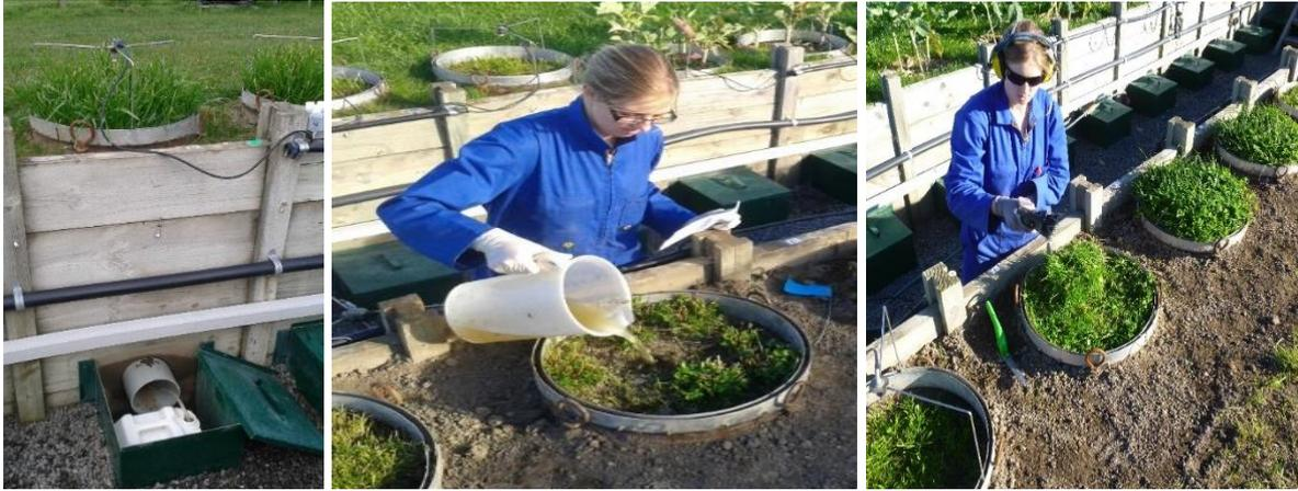
Photos: Left - Lysimeter set-up. Centre - Urine treatment application. Right - Pasture harvest using electric clippers.
