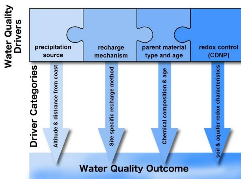
**Figure 1: Conceptual diagram showing the four key drivers of regional hydrochemistry. The drivers identified for Southland are: precipitation source; recharge mechanism; geology and soil age/parent material composition and finally soil and aquifer redox characteristics.**
