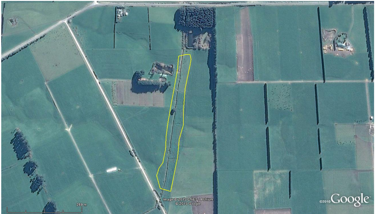
Figure 1: Potential ~3ha constructed wetland site in the upper Waituna Catchment viewed using Google Earth Satellite image. The proposed approximate boundaries of the wetland are shown by the yellow lines
