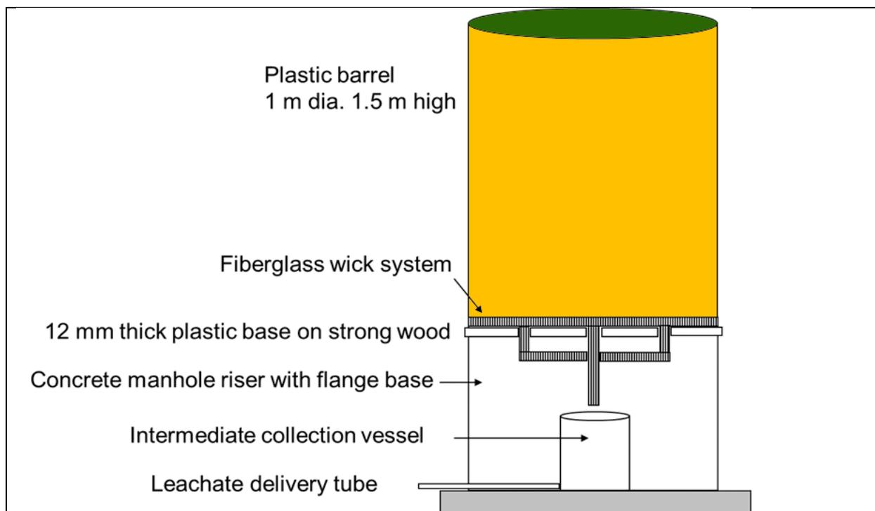
**Figure 1.** Layout of individual lysimeters.
