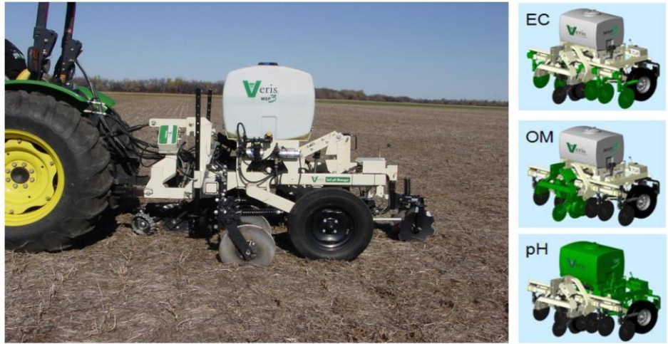
Figure 1. Veris MSP3 Unit, showing components for individual measurements
