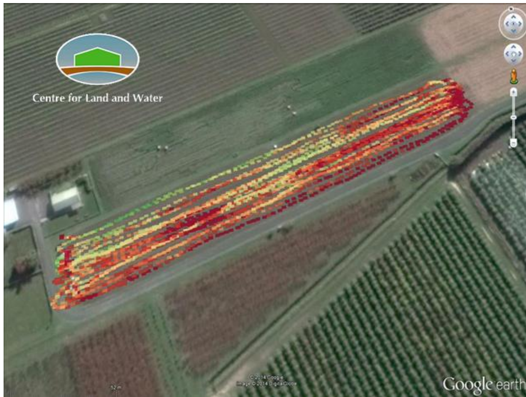
Figure 5 Collected georeferenced data showing onion canopy groundcover percentage three weeks prior to lifting.
