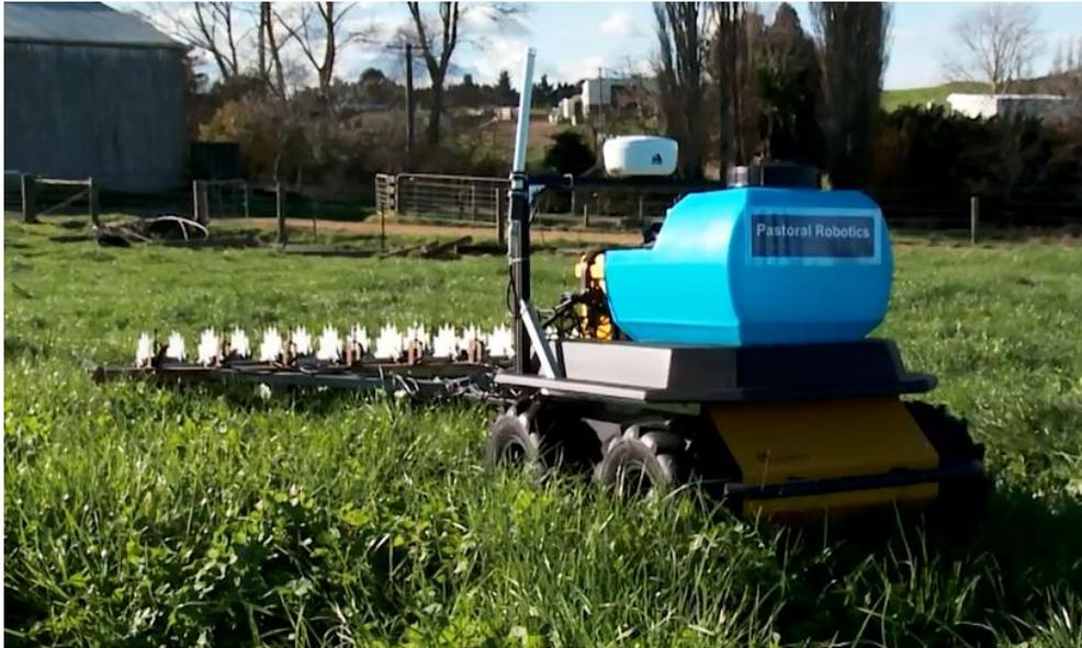
**Figure 8.** The Mini-ME® autonomous robot towing Spikey®.
