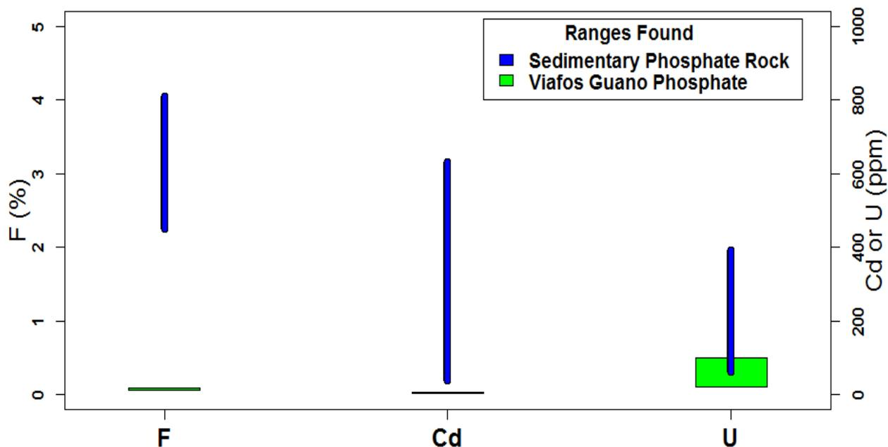
**Figure 1. Contaminant levels in Viafos (Indonesian) Guano Phosphate compared to ranges reported in sedimentary phosphate rocks.**
