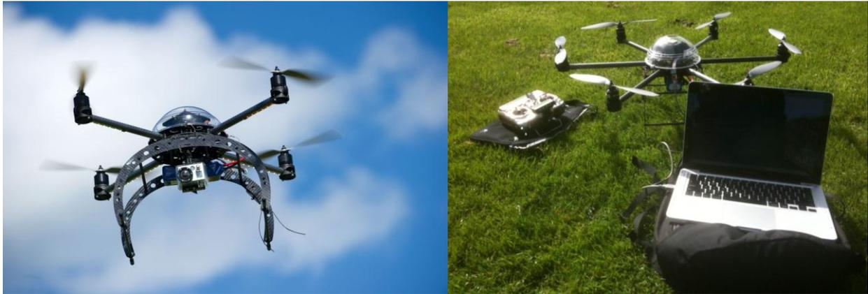
**Figure 1 Left: The QuadKopter carrying a video camera. Right: The HexaKopter on the ground with the remote controller and a laptop to set up the system for a GPS waypoint flight.**
