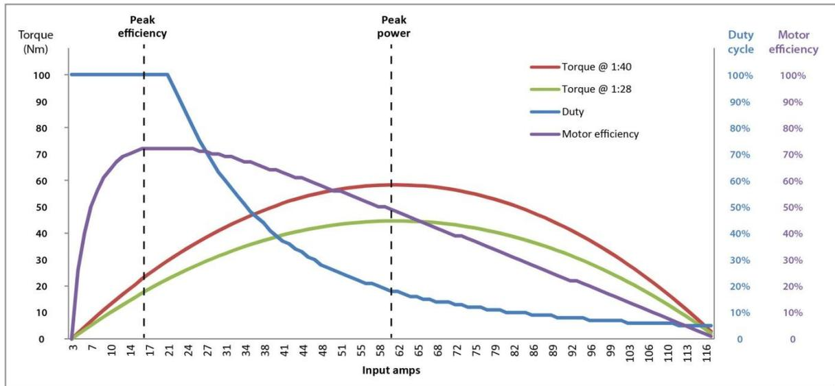
Figure 3: Modelled performance curves for DAGU ME63-066 DC motor with a STM UMI 40 gearbox at 1:40 and 1:28 ratios.
