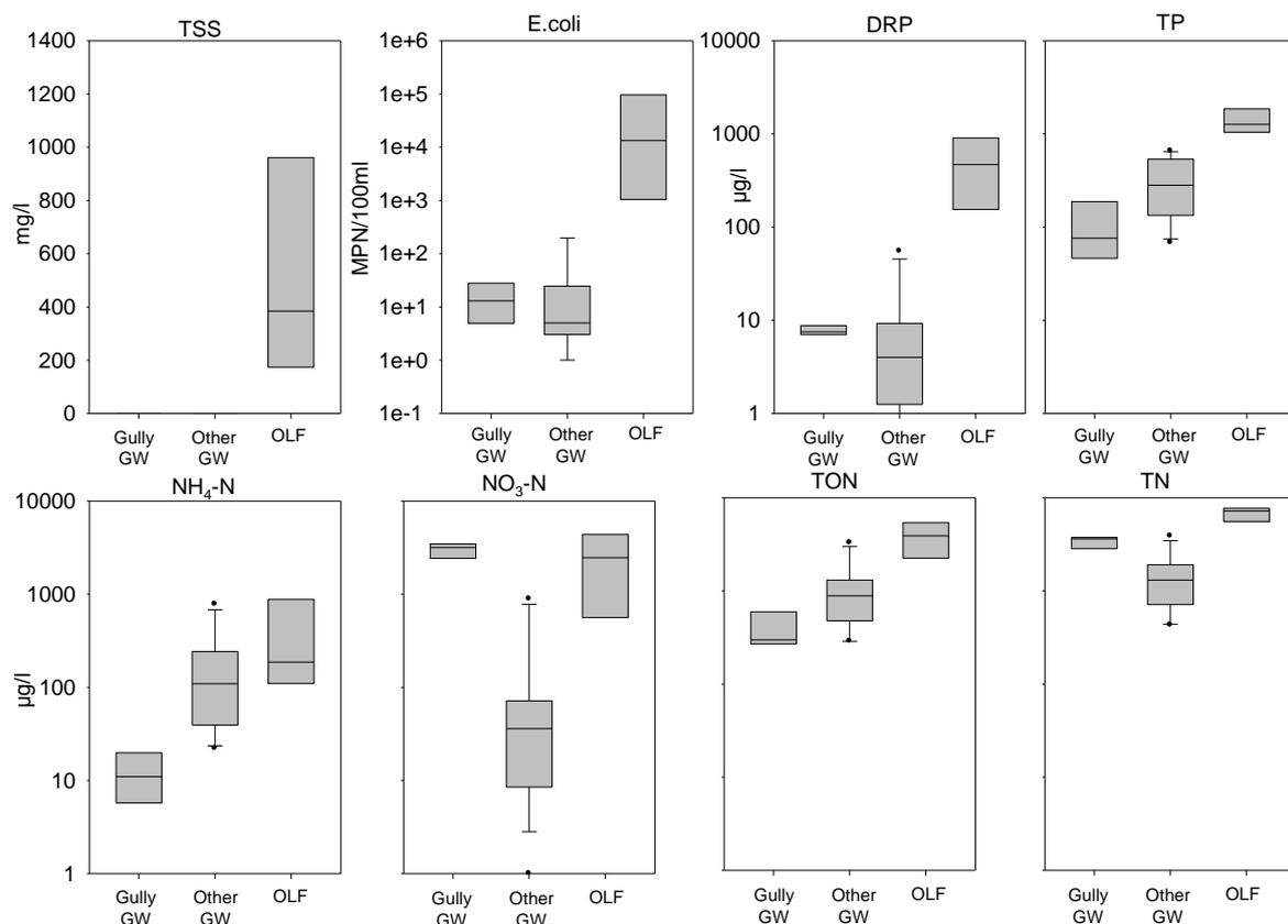
**Figure 6** Box plots of TSS, *E. coli* and different forms of P and N for the gully groundwater, other groundwater locations and overland flow samples (GW = groundwater).
