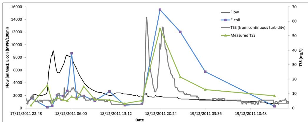
**Figure 9** Flow, *E. coli* and TSS concentrations recorded at the lower weir for the flow and stock access events of 18/12/2011.
