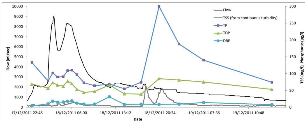
**Figure 11** Flow and concentrations of TSS, TP, TDP and DRP recorded at the lower weir for the flow and stock access events of 18/12/2011.
