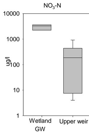
**Figure 5** Box plots of NO<sub>3</sub>-N during baseflow for the wetland subsurface flow immediately upstream of the upper weir and for the upper weir.
