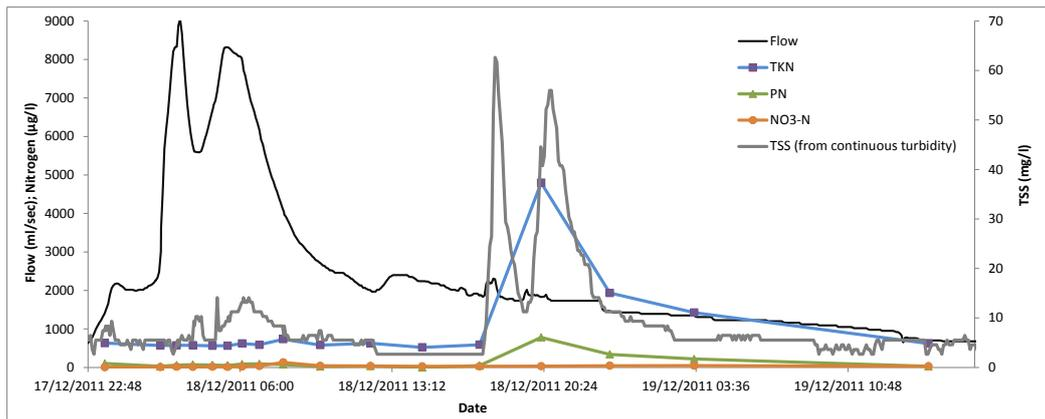
**Figure 10** Flow and concentrations of TSS, TKN, PN and NO<sub>3</sub>-N recorded at the lower weir for the flow and stock access events of 18/12/2011.
