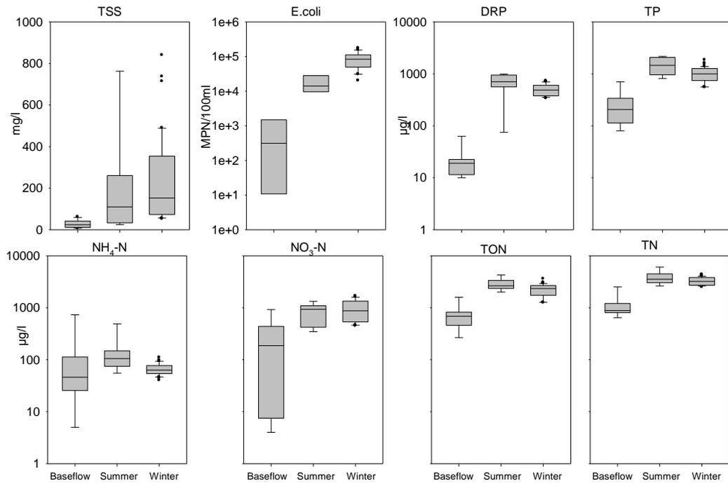
**Figure 3** Box plots of TSS, *E. coli* and different forms of P and N at the upper wetland weir. The box defines the 25th and 75th percentiles and median, whiskers indicate the 90th and 10th percentiles, and outliers are represented by dots.
