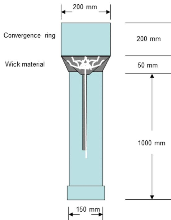
**Figure 1.** Passive wick lysimeter to monitor water and nutrient fluxes.
