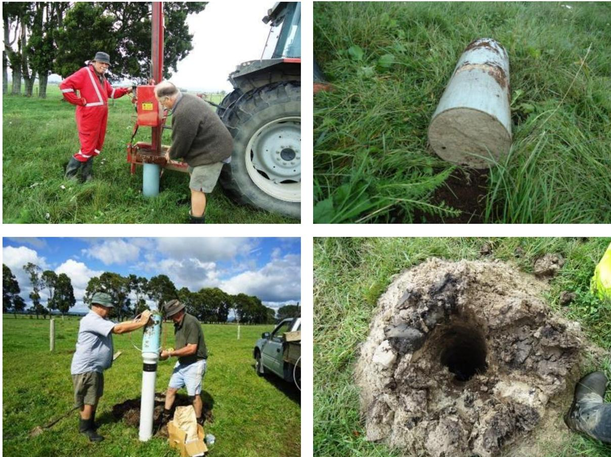
**Figure 2.** Preparation and installation of drainage flux meters
