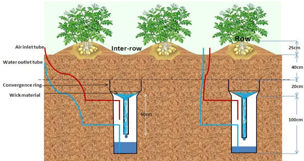
Figure 1. A schematic diagram showing fluxmeters installed under the row (right) and inter-row (left) in the potato field
