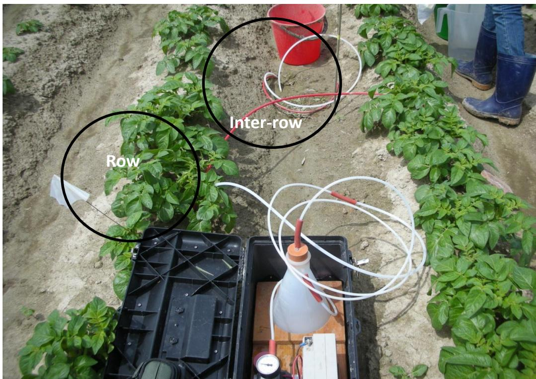
Figure 2 Extraction of drainage by connecting the tube to a pump. Each fluxmeter has two tubes to the surface, the white one to collect the water and the red for air entry and escape.
