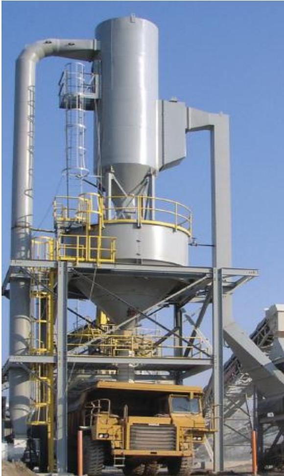
**Figure 2: Shows a Metso static classifier (Source: Metso mining and Construction Ltd.)**
