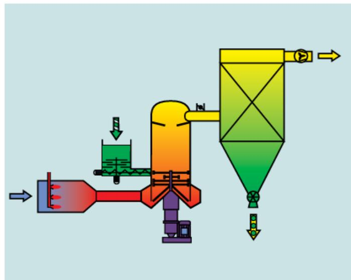
**Figure 4: Shows in line drying by spin flash dryer (Source: Anhydro spin flash dryer [www.spxf.com](http://www.spxf.com))**
