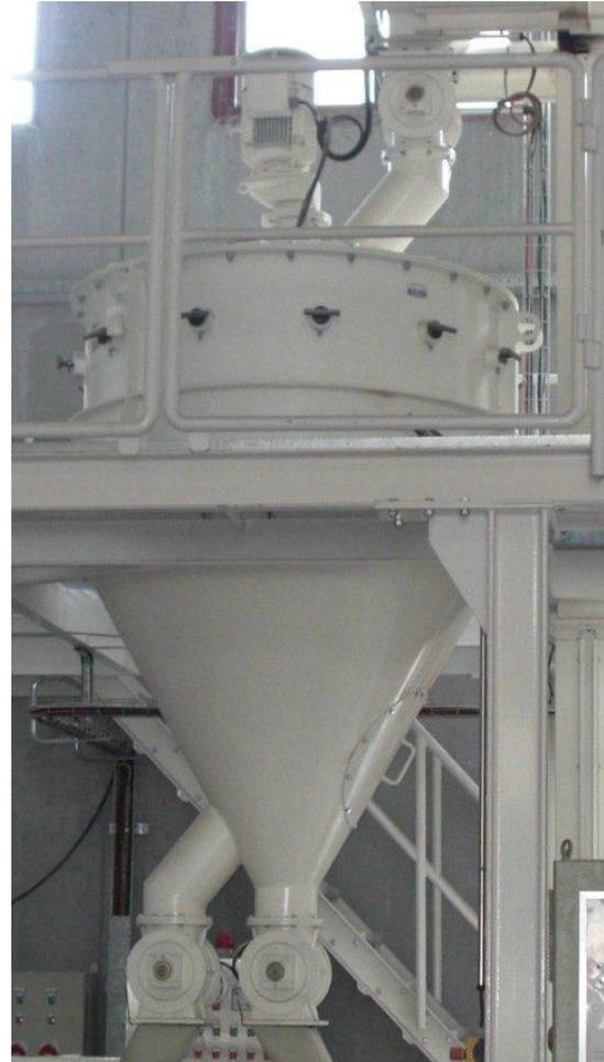
**Figure 3: Shows ULS Dynamic Classifier (Source: Ecutec SL, Catalane , Spain)\_**
