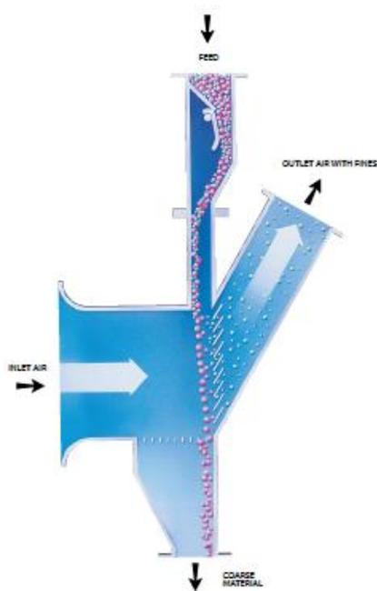
Figure 1a: static air classifier
