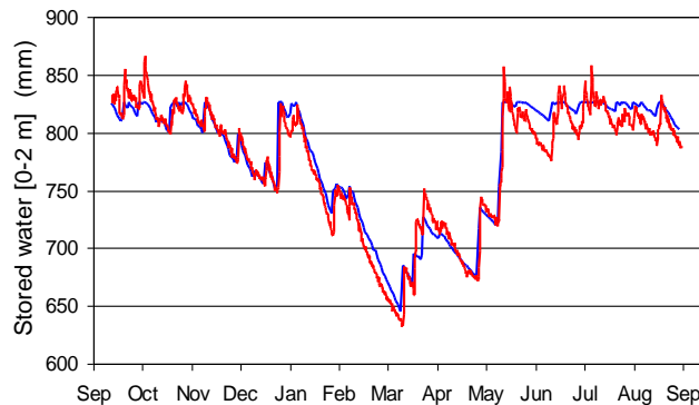
Figure 3. The measured (red) and the SPASMO modelled (blue) storage of water in the rootzone down to 2 m under kiwifruit in the Bay of Plenty.
