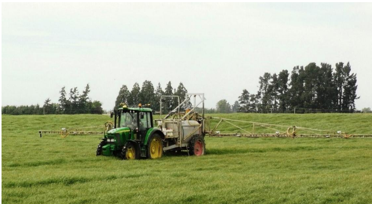
Figure 1. Sensors in use. Cropspec sensors were mounted on the cab of tractor while the Greenseeker and Crop Circle Sensors were mounted on the spray boom as per manufacturer’s instructions.
