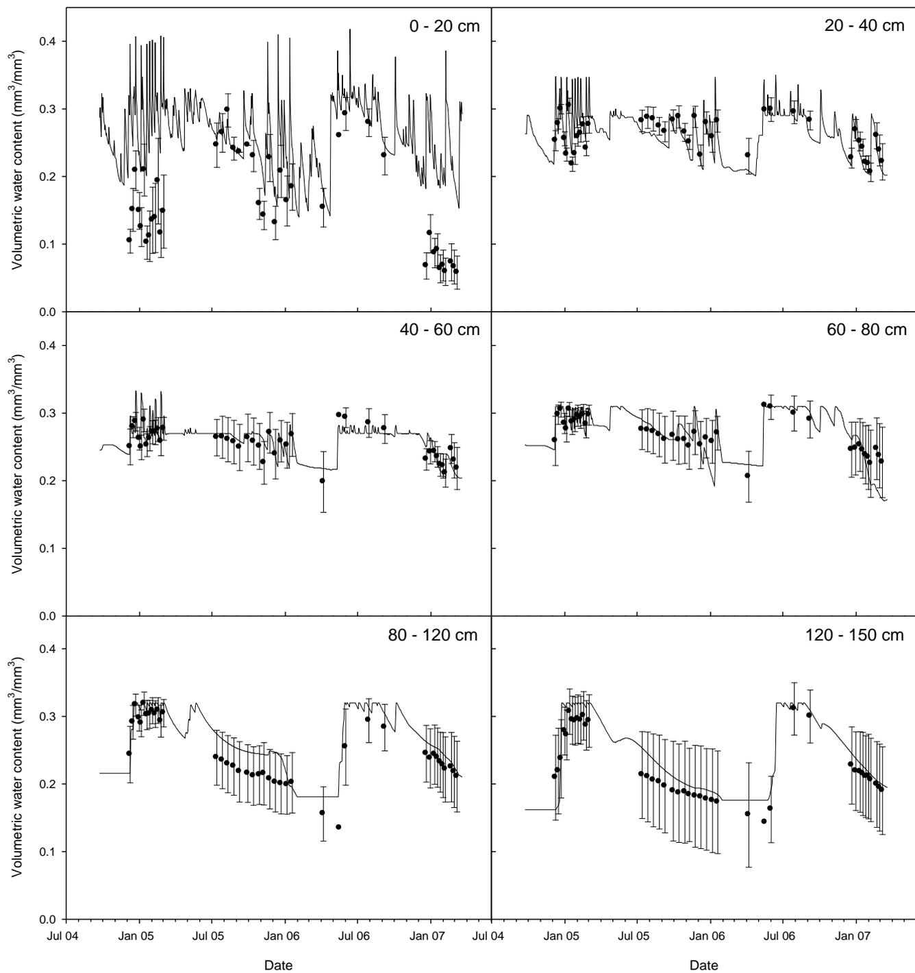
**Figure 3.** Observed (●), with associated standard deviation, and predicted (-) volumetric soil water content through time in soil layers of increasing depth for the W1 treatment.
